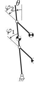
Fig. 3. Inverted pendulum model: The pendulum is stabilized by the relative motion of its two arms.
