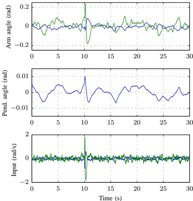
Fig. 4. Typical state and input trajectories for the simulation example. TOP: arm angles  $x_1$  (blue) and  $x_2$  (green). MIDDLE: pendulum angle  $x_3$ . BOTTOM: control inputs  $u_1$  (blue) and  $u_2$  (green). At  $t = 10$ s, an impulsive disturbance is applied on input  $u_1$ .
