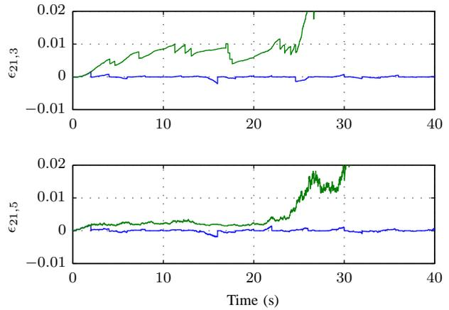
Fig. 6. Two components of the inter-agent error  $e_{21}$  for simulation with synchronous averaging (blue) and without (green). The blue graph is reset to zero at  $t = 2, 4, 6, \dots$  according to (19). Without resetting, the inter-agent errors diverge and destabilize the system.
