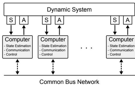
Fig. 1. Networked control system. Multiple control agents (each with an embedded computer, sensors (S) and actuators (A)) are distributed along a dynamic system. Each agent estimates the state of the dynamic system, computes local control inputs, and decides when to communicate with the other units over a common bus network.
