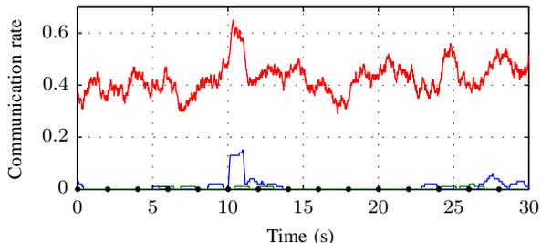
Fig. 5. Communication rates (moving average over 100 steps) for the same simulation experiment as in Fig. 4. The rates are shown in blue and green for the arm angle measurements  $y_1$  and  $y_2$ , and in red for the pendulum angular rate measurement  $y_3$ . The black dots on the time axis indicate the instants when the estimates are reset according to (19).
