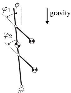
Fig. 3. Inverted pendulum system used for the simulations. The system (confined to the vertical plane) consists of three links: the pendulum, whose angle against the vertical is denoted by  $\phi$ , and two "arms" rotating relative to the pendulum with angles  $\varphi_1$  and  $\varphi_2$ .
