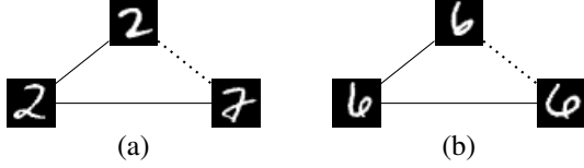
Figure 2: Examples of inconsistent edge labels produced by a stand alone Siamese network on the MNIST digits.
