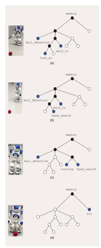
Figure 2. Some possible patterns of activation of the tree presented in Figure 1 where the robot is (a) walking toward the ball when it sees it; (b) walking toward the last known position of the ball while searching for it with its head; (c) performing a full body search; and (d) sitting in a safe position when its battery runs low. Black is used to indicate activation of nodes and blue activation of leaf nodes. For brevity, only activated leaf nodes are labeled.
