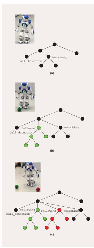
**Figure 4.** An illustration of dynamic topology updating. (a) The topology of the behavior tree at runtime prior to any ball detection by the robot. (b) The robot detects a green ball, and a corresponding following subtree is instantiated (in green). (c) A red ball is detected, resulting in the instantiation of a competing following subtree (in red).
