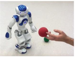
Figure 6. A Nao robot executing the ball-grouping behavior.
