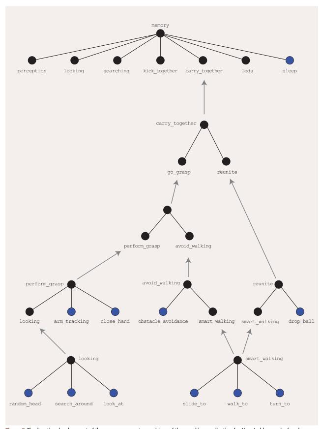
Figure 7. The iterative development of the <code>carry\_together</code> subtree of the reuniting application for Nao. In blue are leaf nodes. From bottom to top, trees of small size are created and debugged and then used as leaf nodes of trees of higher levels of abstraction. Other nodes of the full application, e.g., <code>kick\_together</code>, are developed using a similar approach (but are omitted here for brevity).
