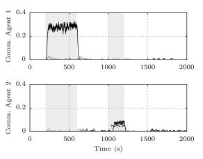
**Fig. 5** Event-based communication rates for the thermo-fluid simulation example: communication of level measurements  $y_{11}$  and  $y_{21}$  in black (dotted), for temperature measurements  $y_{12}$  and  $y_{22}$  in black (solid), and for the inputs  $u_1$  and  $u_2$  in grey. Communication rates are computed as the moving average over 100 steps (0.0 meaning no communication and 1.0 full communication)
