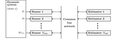
**Fig. 1** Distributed state estimation problem. Multiple distributed sensors make observations  $y_i$  of a dynamic system and communicate to estimator nodes via a common bus network. Development of an event-based scheme allowing all estimators to estimate the full system state x, but with limited inter-agent communication, is the objective of this paper
