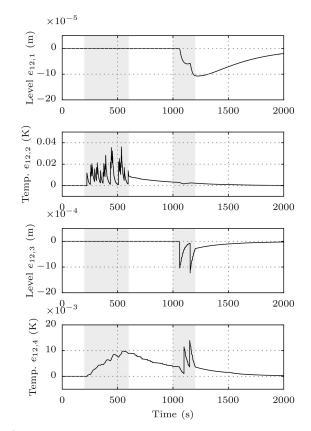
**Fig. 6** Inter-agent error  $e_{12}$  for the thermo-fluid example. Jumps in error are caused by packet drops, and the decay afterward is due to stable interagent dynamics (29) as ensured by Lemma 1
