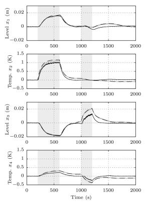
**Fig. 4** State trajectories for the thermo-fluid simulation example. Black (dashed): the actual states x; black (solid): event-based estimate  $\hat{x}_1$  by Agent 1; grey: centralised estimate  $\hat{x}_c$ . Centralised estimate is shown for comparison and not available on any of the agents. Grey shaded areas indicate periods where step-wise process disturbances are active
