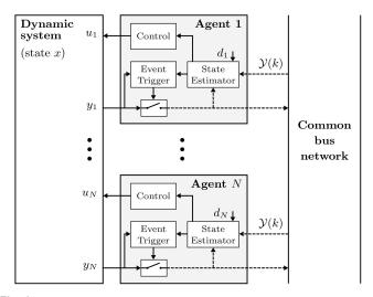
**Fig. 3** Distributed, event-based control architecture in the experiments of Section 6. N spatially distributed agents observe and control a dynamic system and exchange data with each other via a common bus. Compared to Fig. 2b, the agents combine the functions of sensing/triggering, estimation, and additionally feedback control. The State Estimator serves both for making the triggering decision and for feedback control
