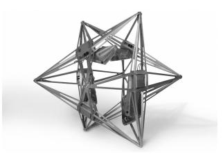
**Fig. 7** The Balancing Cube [31] can balance autonomously one any one of its corners or edges. Six rotating arms, which constitute the control agents, collaboratively keep the system in balance. Here, the cube is shown while balancing on an edge, which was the configuration used for the experiments in [3]. Photo: Carolina Flores, IDSC, ETH Zurich. © 2012 IEEE. Reprinted, with permission, from [31]
