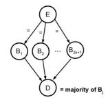
redundancy code: bit E is copied to all  $B_i$
