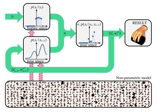
**Fig. 2.** Schematic figure of the non-parametric temporal pose estimation framework. Given an image observation  $\mathbf{y}_t$ , a set of pose hypotheses  $\mathbf{X}_t$  are drawn from the model. Each hypothesis is given a temporal likelihood based on consistency with the hypothesis in the previous frame. The final estimate is the pose associated with the largest probability.
