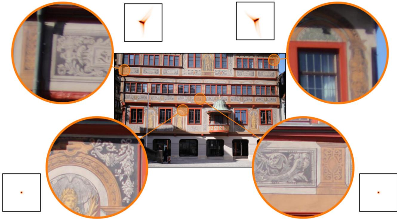
Optical aberrations can be characterised by the *point spread function* (PSF)
