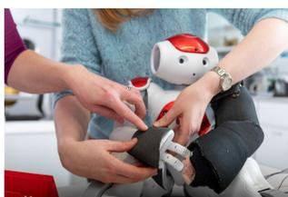
Building a sensor flat and then wrapping it around a surface degrades sensitivity. Instead, the sensor is fabricated along a curvature matching that of the robot's body part.
