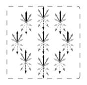
Figure 6-13: Each arrow cluster is a MT subunit where the pattern direction is computed using a WIM model[135]. A MT cell is modeled by the set of nine clusters equally distribute within its receptive filed, and the response is obtained by summing the responses of the 9 clusters. Reprinted from [137].
