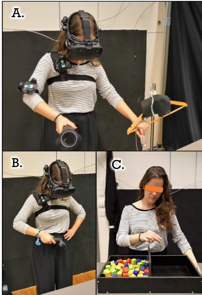
FIGURE 3.2: A participant in the setup of the pilot experiment. **A.** During an inverse kinematics trial, wearing a shoulder tracker, an elbow tracker, and a pulse oximeter. **B.** Subjects from the prosthesis mimicking group did not have to wear an elbow tracker, and half of the participants ran the experiment without using oximetry. **C.** The real box and blocks test, standing as in VR.
